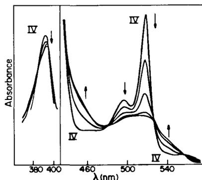
FIG. 1. Titration of  $\text{Ru}^{\text{II}}(\text{MplIX})(\text{DMF})_2$ , **IV**, with aliquots of  $\text{Br}_2/\text{DMF}$  to give  $\text{Ru}(\text{III})$  species (directions of arrows indicate changes in spectra as  $\text{Ru}(\text{II})$  is consumed).
