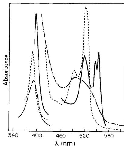
FIG. 3. Absorption spectra of ruthenium myoglobins in aqueous phosphate buffer, pH 8.0. Ru<sup>III</sup>Mb, ····; Ru<sup>II</sup>Mb, ---; Ru<sup>II</sup>(CO)Mb, —.
