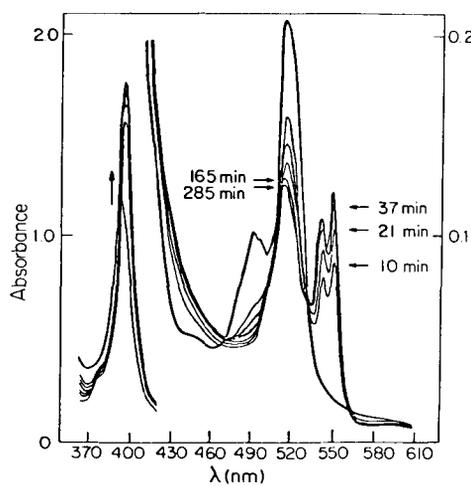
FIG. 4. Reaction of Ru<sup>II</sup>Mb with 1 atm of CO at 0°C to form Ru<sup>II</sup>(CO)Mb; spectra as a function of time (cf. Fig. 3).
