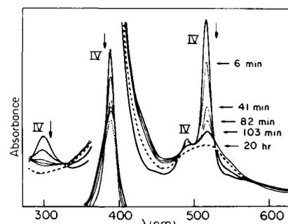
FIG. 2. Oxygenation (1 atm of  $\text{O}_2$ ) of  $\text{Ru}^{\text{II}}(\text{MplIX})(\text{DMF})_2$ , **IV**, in DMF at  $0^\circ\text{C}$  to give  $\text{Ru}^{\text{II}}(\text{O}_2)(\text{MplIX})(\text{DMF})$ . The spectrum at 20 h (---) shows irreversible oxidation to  $\text{Ru}(\text{III})$ .
